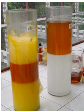
Left: crude palm biodiesel wash. Right: WVO, sunflower biodiesel wash.
